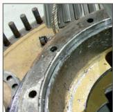
Pitting on bearing
