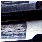
Abrasion on gear
